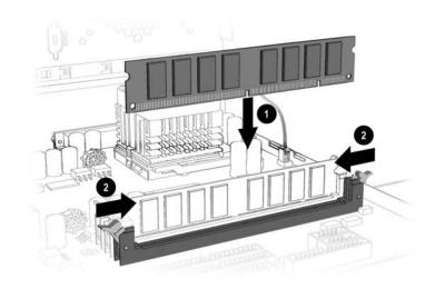
**Note:** Press gently to ensure the memory module is properly positioned.
